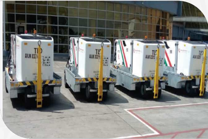
4 new Ground Power Units (GPU)
